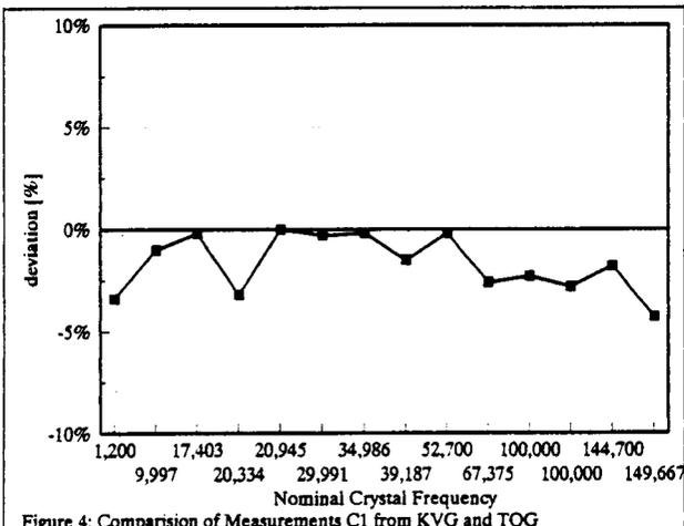
Figure 4: Comparison of Measurements C1 from KVG and TQG
