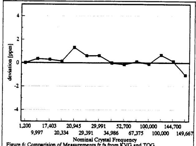
Figure 6: Comparison of Measurements fr.fs from KVG and TQG
