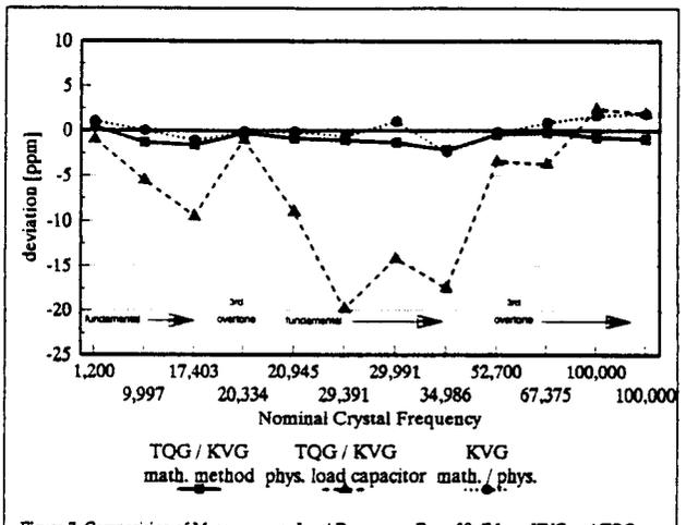
Figure 7: Comparison of Measurements Load Resonance Freq. 30pF from KVG and TQG
