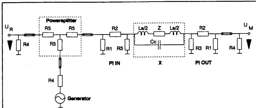
R1: 159 Ohm, R2: 66.2 Ohm, R3: 14.2 Ohm, R4: 50 Ohm, R5: 50/3 Ohm
