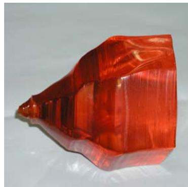
As the piezoelectric coupling factor is 2.3 to three times that of quartz, resonators with high pullability can be manufactured with this material, having a temperature stability and a Q-factor, which are in the same order of magnitude as those of quartz resonators.
