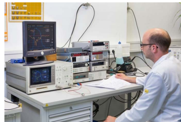
Electrical testing of oscillators
