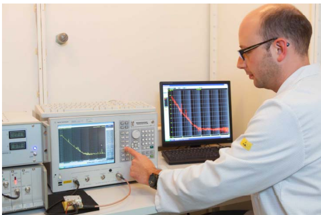
Phase noise test systems in shielded cabinet
