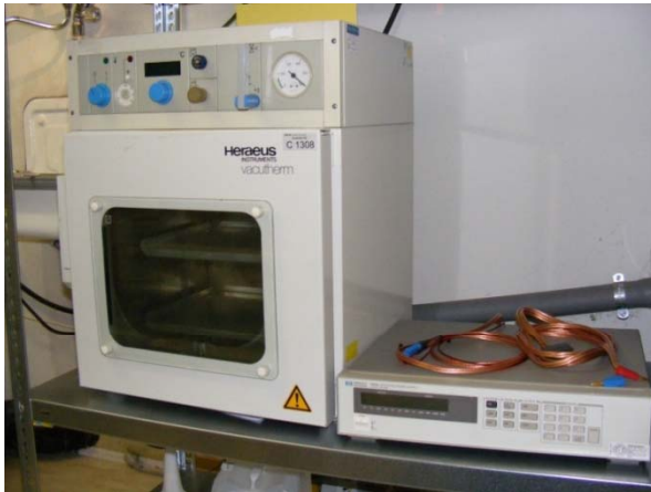
Burn-in test under vacuum
