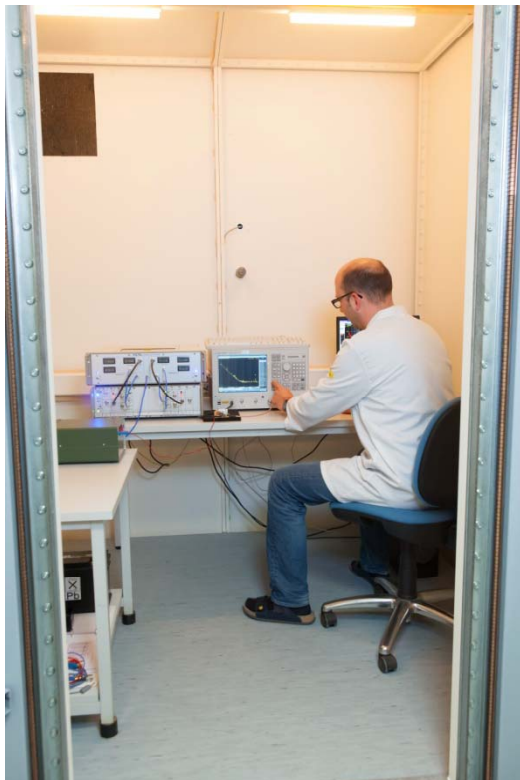
Phase noise test in shielded cabinet
