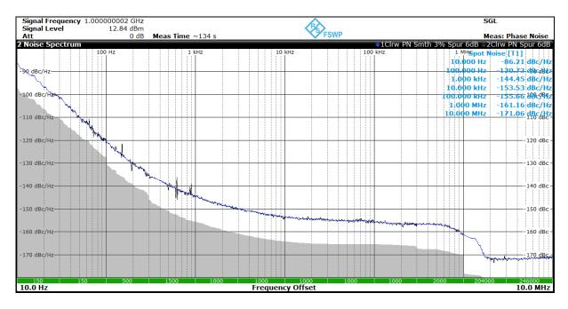
(3) 1.3 GHz Output (Multiplication x10 including SAW Filter) Locked to Ultra-Low Noise 10 MHz Reference for ultra-low jitter
