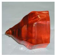
As the piezoelectric coupling factor is 2.3 to three times that of quartz, resonators with high pullability can be manufactured with this material, having a temperature stability and a Q-factor, which are in the same order of magnitude as those of quartz resonators.
